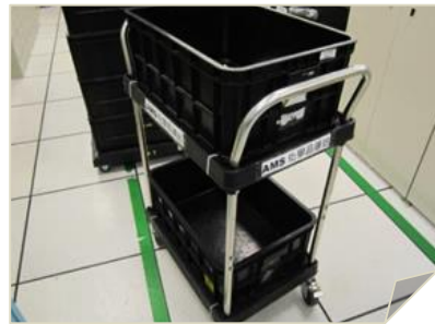
Set up chemical material acquisition truck to avoid turnover during transport
